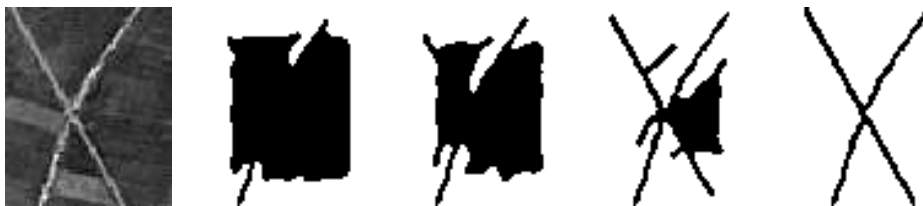
Figure 2.4: Road detection on a SPOT satellite image. Left: Original image; four rightmost: evolution. Image ©French Space Agency (CNES) (Rochery et al., 2005c).
