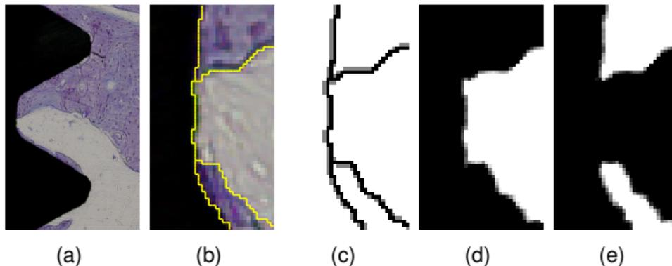
**Figure:** (a): The screw-shaped implant (black), bone (purple) and soft tissue (light grey). (b) Part of a crisp (manual) segmentation of (a). (c) The set of re-evaluated pixels. (d) and (e) Pixel coverage segmentations of the soft tissue and the bone region, respectively.
