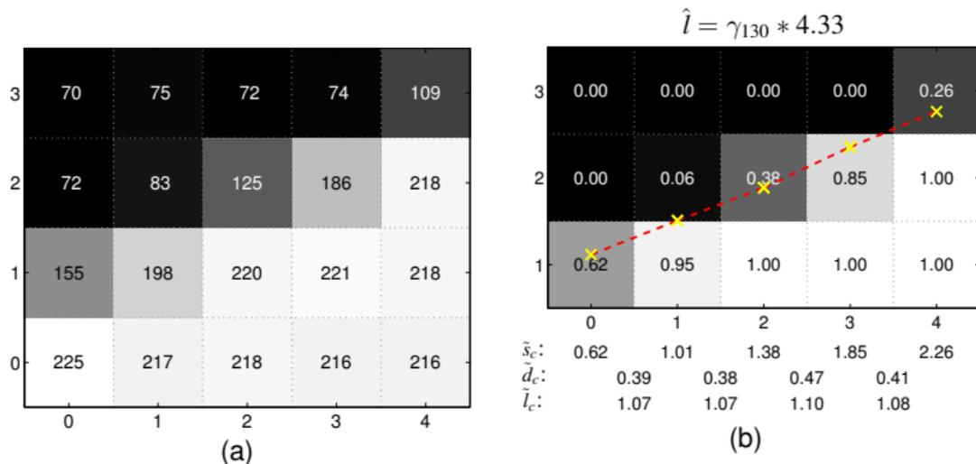
**Figure:** (a) Close up of the straight edge of a white paper imaged with a digital camera. (b) Segmentation output from Algorithm 2 using 130 positive grey-levels. Approximating edge segments are superimposed.
