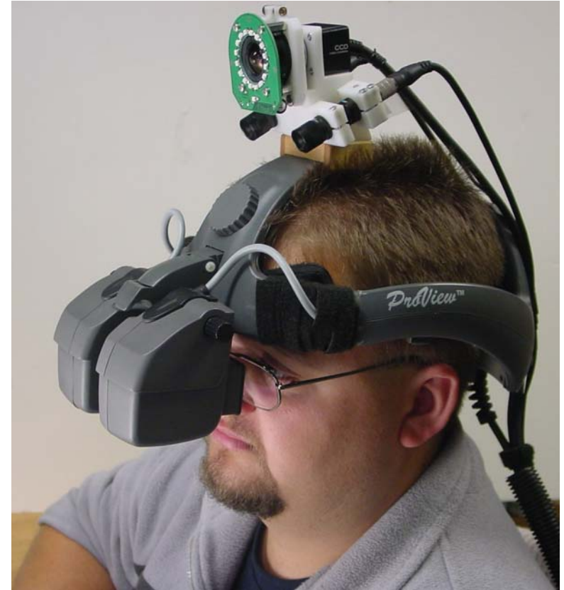
A head-mounted video see-through display. Photograph courtesy of Dr. Frank Sauer, Siemens Corporate Research, Princeton/NJ.
